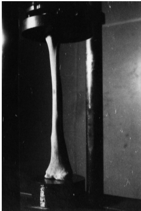
Figure 7. Photograph from the IL archive showing a compressive strength test of an animal bone; 1970s–1980s (ILEK Archive).
